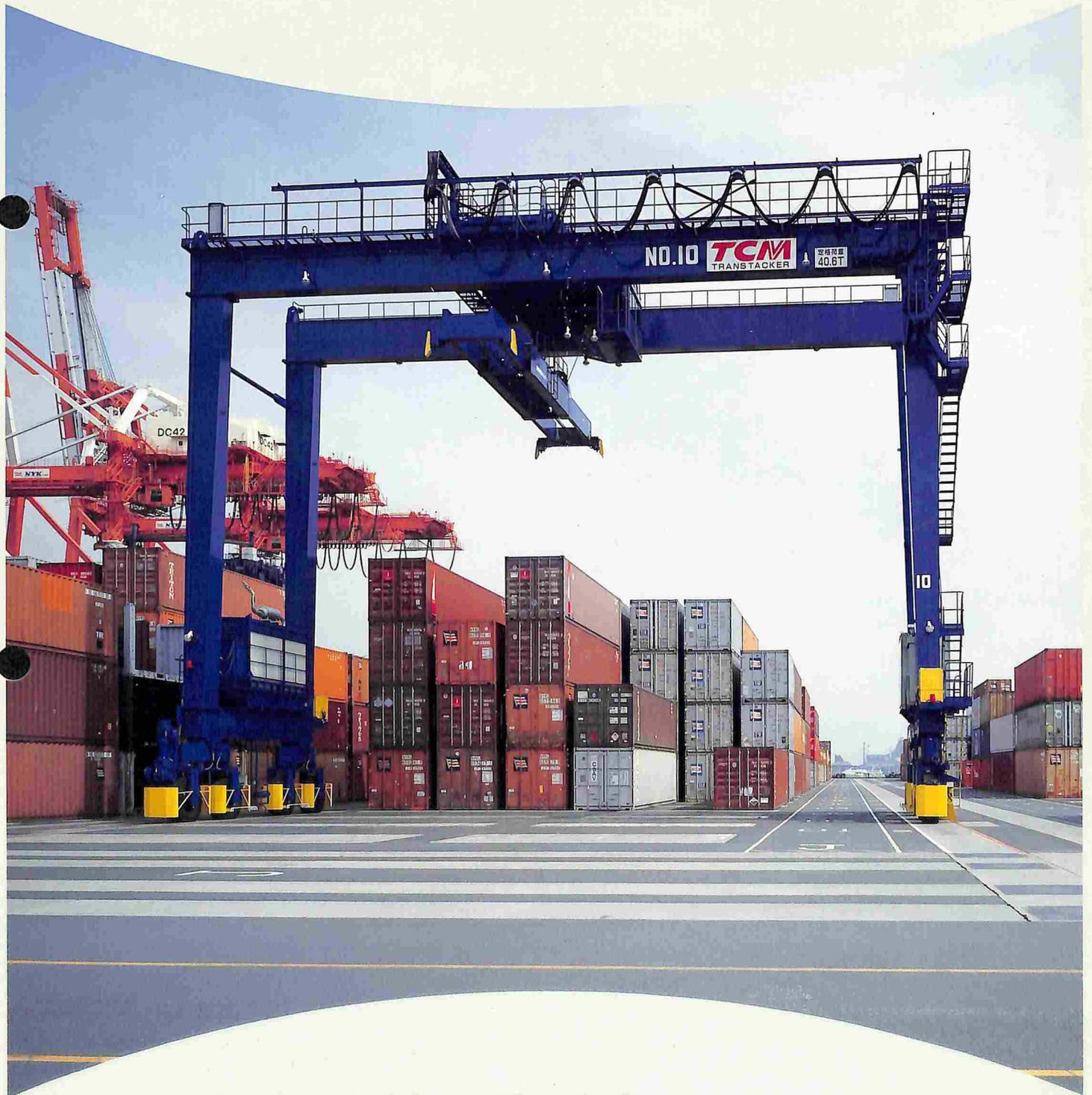
RTG (Rubber Tired Gantry crane)
