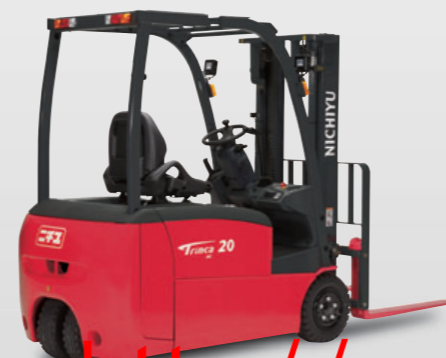
Photo: FBT20PN (L2) series long wheel base and large battery, "L2" series
